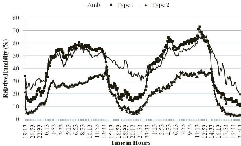
Figure 3. Relative humidity in Type 1 and Type 2 dryers and ambient condition (Without loading potato slices from 12 to 14 May 2010).
